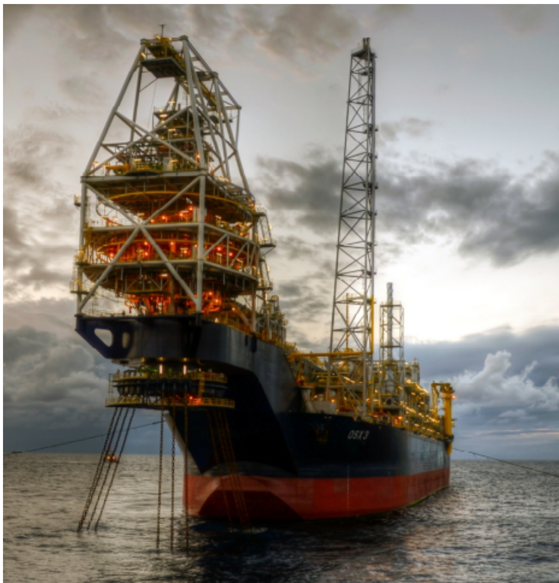
Figure 1 - FPSO BRAVO turret system
