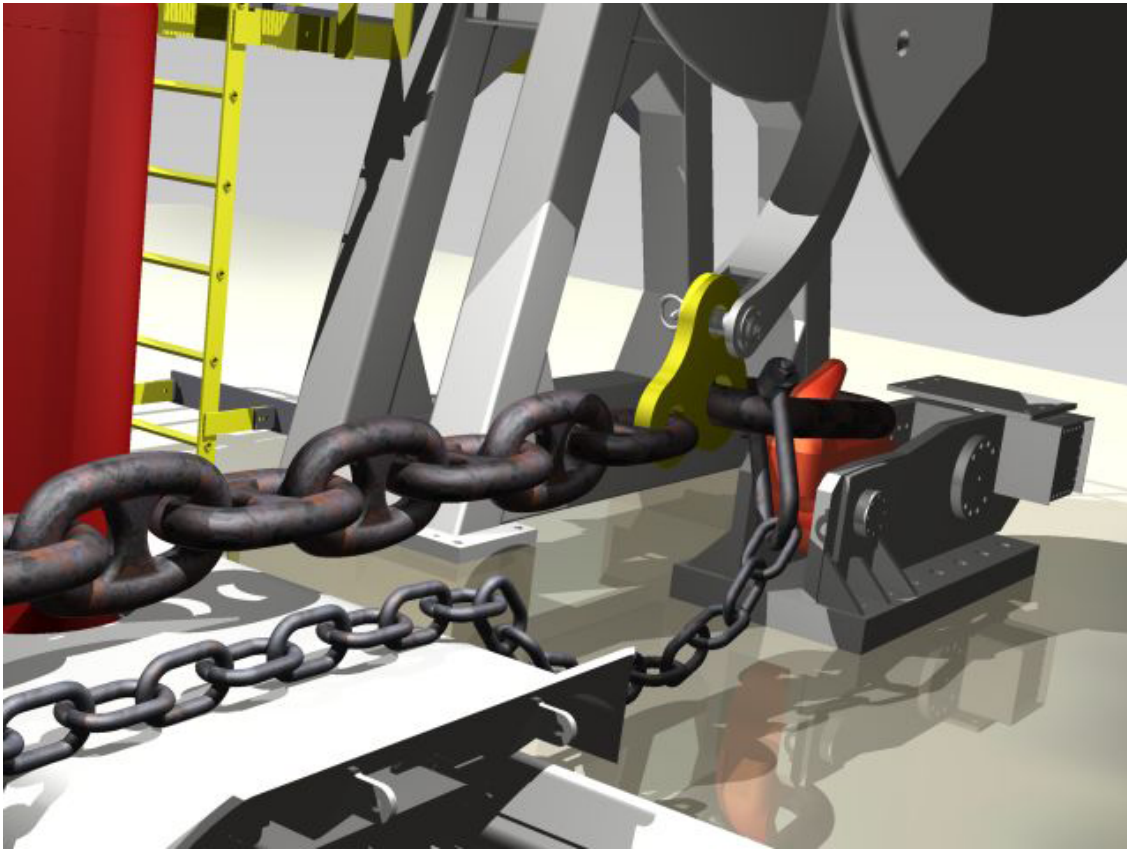
Figure 6 - Detail of FPSO QRH (Quick Release Hook)
